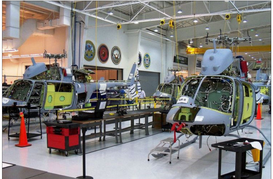
Northrop Grumman MQ-8C Fire Scouts on the assembly line in Moss Point, Miss.
