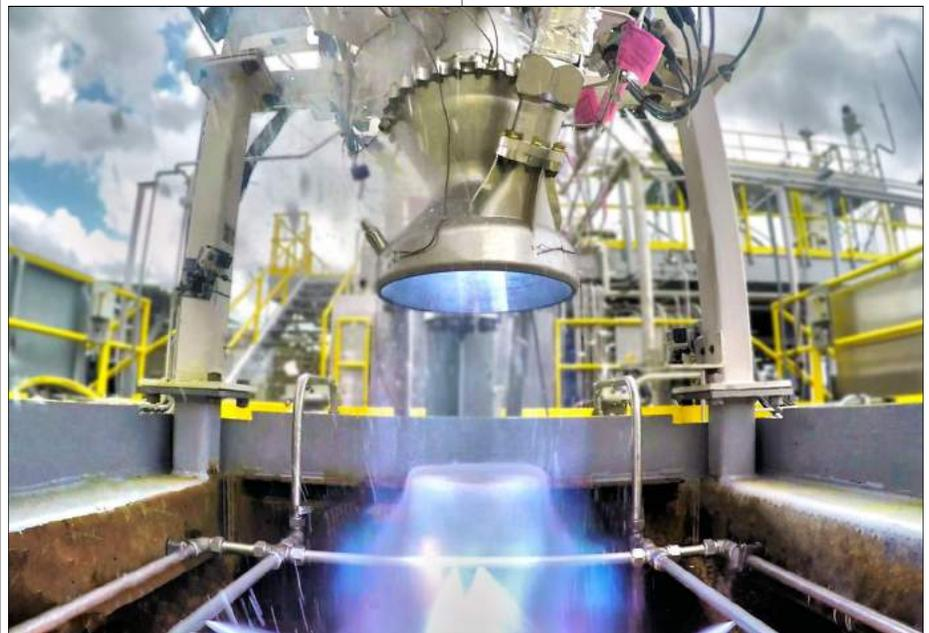
Test of Aeon 1 rocket engine being developed by Relativity.
