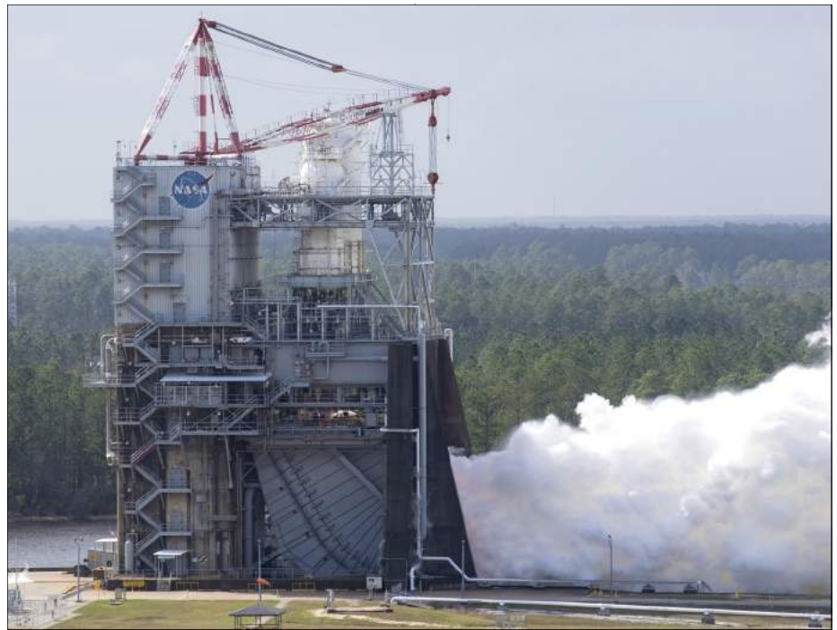
February 2018 full-duration test of RS-25 on the A-1 test stand.
