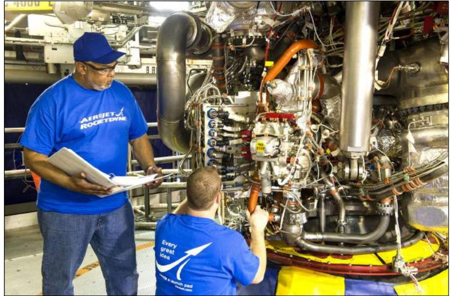
Aerojet Rocketdyne technicians check new RS-25 controller.
